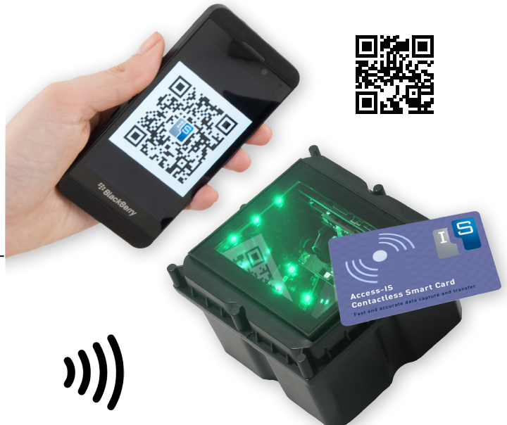
The LSR118 will read a 2D barcode or NFC tag on a smartphone or contactless smart cards.
